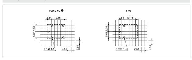
**①** Set of two normally open contacts with a common connection for the moving contact. **②** In case of no tolerance shown in outline dimensions: outline dimension  $\leq 1 \text{ mm}$  tolerance  $\pm 0.2 \text{ mm}$ ; > 1 mm and  $\leq 5 \text{ mm}$  tolerance  $\pm 0.3 \text{ mm}$ ; > 5 mm tolerance  $\pm 0.4 \text{ mm}$ .
