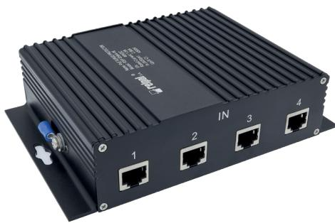
PoE surge protector is designed for protecting Gigabit Ethernet and Power over Ethernet (PoE) terminals or RJ45/Ethernet cable system against surges. Is fulfilling the requirements of Category 6 & all version of PoE (PoE+, PoE ++), can be universally used for all data services with nominal voltages up to 65V. It is ideally suited for PoE and Gigabit Ethernet application and similar applications in structured cabling systems.
