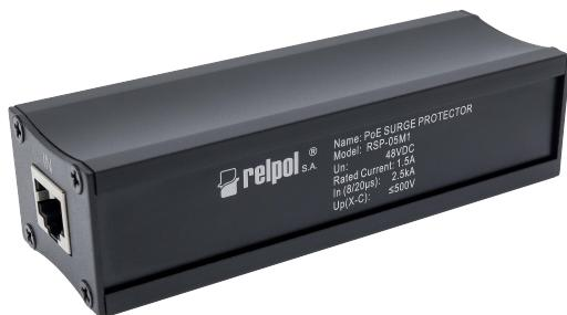
PoE surge protector is designed for protecting Gigabit Ethernet and Power over Ethernet (PoE) terminals or RJ45/Ethernet cable system against surges. It is fulfilling the requirements of Category 6 & all version of PoE (PoE+, PoE++), can be universally used for all data services with nominal voltages up to 65V. It is ideally suited for PoE and Gigabit Ethernet application and similar applications in structured cabling systems.
