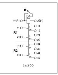
**①** The control terminal S is activated by connection to A1 terminal via the external control contact S.
