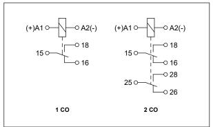
$\mbox{\bf Note}:$  the indicated polarization of the supply refers only to the relays RPC-...-UNI.
