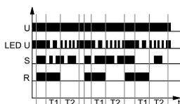
The input of the time relay is supplied with voltage U continuously. Closing of the control contact S switches on the output relay R. Opening of the control contact S starts the interval T1, and after the interval has
