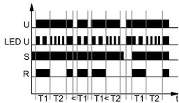
When the control contact S is closed, application of the supply voltage U starts operation in the NWu function - from switching on the output relay R for the interval T1, and after the interval T1 has lapsed, the output relay switches off for the interval T2, and following the interval T2, the output relay R switches on for continuous time.
