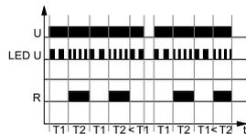
Application of the supply voltage U when the control contact S is open start the cyclical operation in the Ip function - from the interval T1 (time of switching off the output relay R), following which the output relay R is switched on for the interval T2. The cyclical operation continues until the supply voltage U is interrupted.
