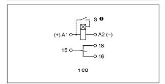
$\pmb{\theta}$  The control terminal S is activated by connection to A1 terminal via the external control contact S.
