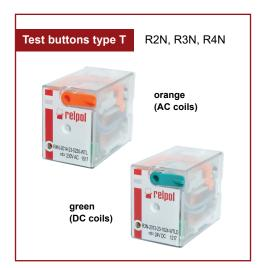
**Test buttons (no latching)** are recommended for R2N...WT, R3N...WT, R4N...WT, R15...WT 2 CO, R15...WT 3 CO relays - **for applications that do not allow permanent contact latching**. By manual operation (pressing the button) relay contacts can get switched for as long time as long the button is pressed. Contacts return to initial position as soon as pressure is released from the button. Those operations can be done while the coil is deenergized **(6)**.
