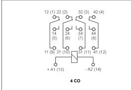
Note: the indicated polarization of the supply refers to the relays with extra equipment  ${\bf D}$  - surge suppression element (diode) - for DC coils only.
