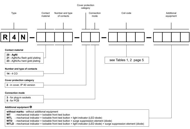
3 T - orange colour (AC coils), green (DC coils). WT - standard equipment of relays. WTD, WTLD - available only in relays with DC coils.
