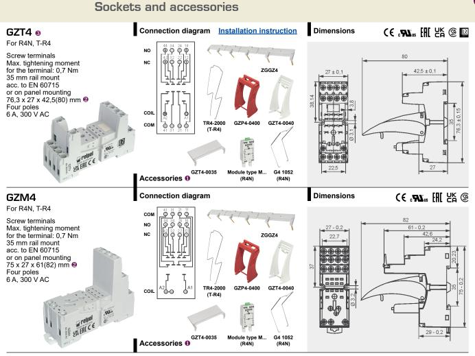
Image: Mounting and sub-assemblies of accessories in the socket - see page 9. Signalling / protecting modules type M... - see page 12. In the bracket the height of socket with retainer / retractor clip is shown. 8 Have obtained LR Type Approval Certificate (Lloyd's Register).
