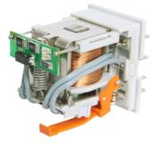
Application of electronics made in the SMD technology: additional equipment L (LED diode) and D (diode) are located on the printed circuit board; the change of the position of the LED diode and optimization of the quality and intensity of its light provide certainty that the relay is in operation status when the LED is on.
