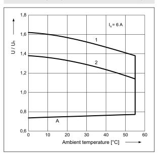
${\bf 1},\,{\bf 2}$  - values on Y axis represent allowed overvoltage on coil at certain ambient temperature and contact load:
