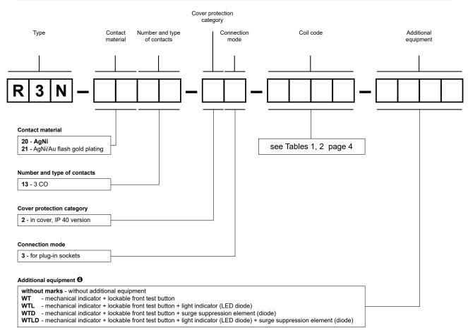
T - orange colour (AC coils), green (DC coils). WT - standard equipment of relays. WTD, WTLD - available only in relays with DC coils.
