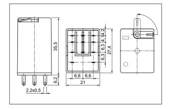
**Dimensions** - plug-in version, with test button (no latching) or with plug (no manual operation)
