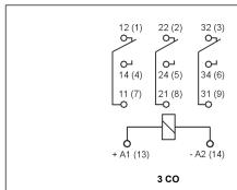
Note: the indicated polarization of the supply refers to the relays with extra equipment **D** - surge suppression element (diode) - for DC coils only.
