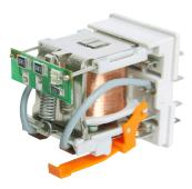
Application of electronics made in the SMD technology: additional equipment L (LED diode) and D (diode) are located on the printed circuit board; the change of the position of the LED diode and optimization of the quality and intensity of its light provide certainty that the relay is in operation status when the LED is on.
