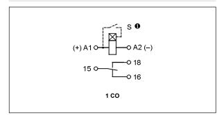
$\boldsymbol{0}$  The control terminal S is activated by connection to A1 terminal via the external control contact S.
