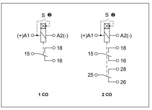
**Note**: the indicated polarization of the supply refers only to the relays RPC-...-UNI. **2** The control terminal S is activated by connection to A1 terminal via the external control contact S.
